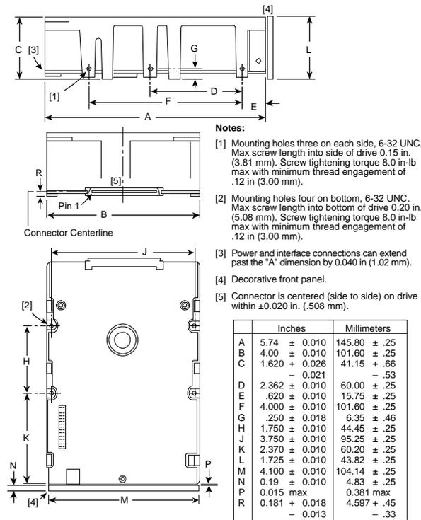
**Figure 6. Mounting configuration details for ST11200NC model drives**
