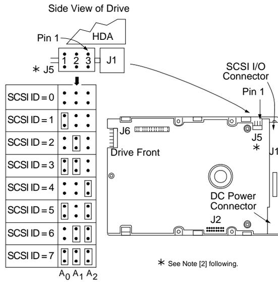
Figure 3b. Drive configuration for ST11200 family
