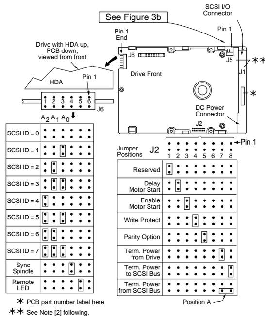
Figure 3a. Drive configuration for ST11200 family
